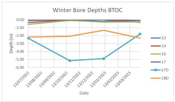
**Figure 8:** Depth of winter storage bores at Gadara Park in meters below top of casing (BTOC)
