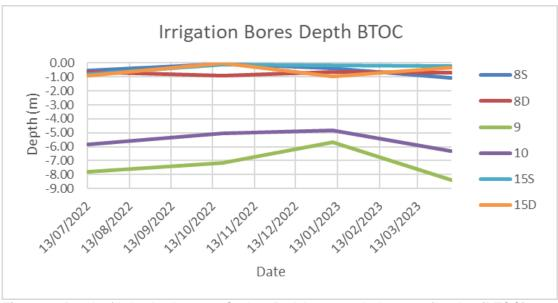
Figure 7: Depth of irrigation bores at Gadara Park in meters below top of casing (BTOC)
