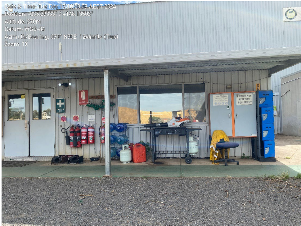
Photo 1 – Two jerry cans and a gas bottle stored together in an area not bunded.
